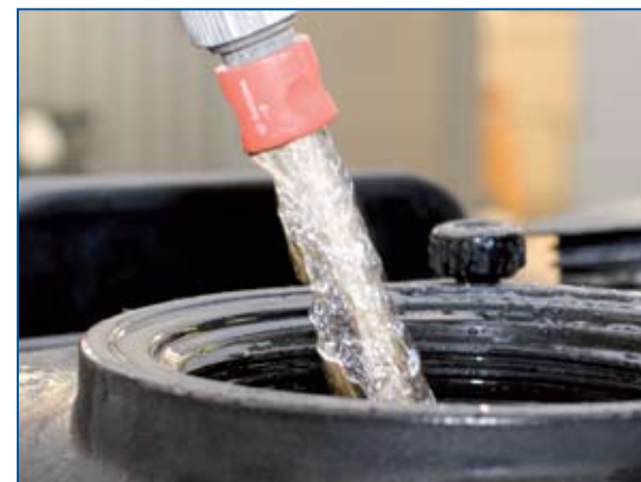
3. Use 1/2 of the normal dilution of neutral cleaner when filling the tank
